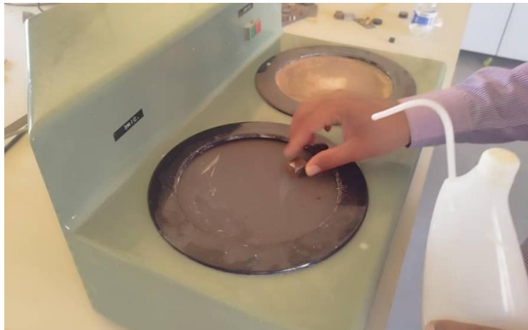
Fig. 4: Metallographic surface preparation (grinding) of the steel specimens.
