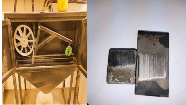
Fig. 6: Wear pattern on specimen surface after abrasion test.
